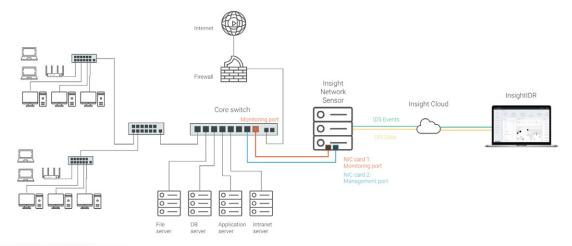
Figure 1: An example deployment of the Insight Network Sensor. A SPAN or mirror port is configured at the network core, which allows the capture of any traffic passing through (both north-south and east-west).
